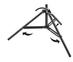
3 Loosen the lower screw knob. Then extend the center column to the length you want.
